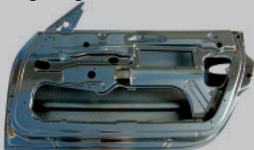
Lightweight Carbon Doors incl. sidebar protection
